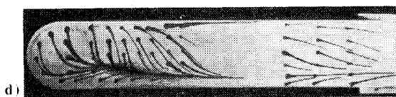
Fig. 16 Surface streaks in disassembled model. a) Axial view from inlet side; b) View of centerbody, outlet to left; c) View into ring towards inlet tube. Outlet and splitter plate to right; d) splitter plate, from left to right.
